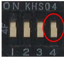
Move down the pin#4 of the Function Select Switch, and the mode is PC Configuration mode.
