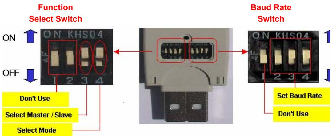
Set the Mode with pin #4 of Function Select Switch.
