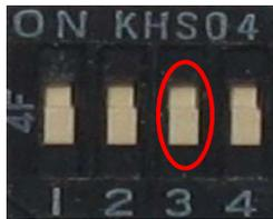
Move down the pin #3 of the function selection switch, to work as SLAVE.
