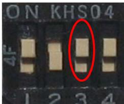
Move up the pin#3 of the function selection switch, to work as MASTER.
