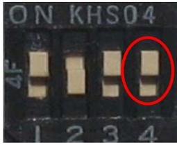
Move Up the pin#4 of the Function Select Switch, and the Mode is DIP Switch mode.
